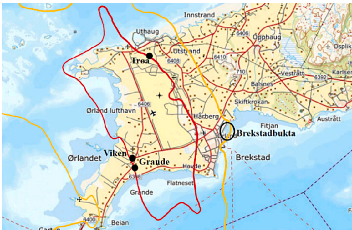
Fig. 2.1. Part of Ørlandet Municipality, showing Ørlandet and Brekstad. The red line represents the red noise zone, and the yellow line represents the yellow noise zone. The current location of the three assessed farmhouses (Trøa, Grande and Viken) and the recently designated Brekstad Bay (Brekstadbukta) area are also indicated. Drawn on the map from norgeskart.no . (For interpretation of the references to colour in this figure legend, the reader is referred to the web version of this article.)
