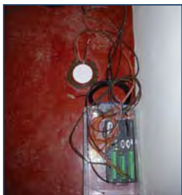
Thermal testing equipment installed above and below concrete floor.
