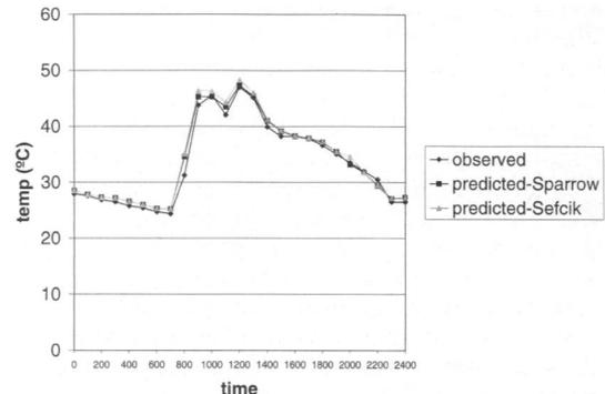
Figure 8 Observed versus predicted temperatures for surface 1 for vented protective glazing.
