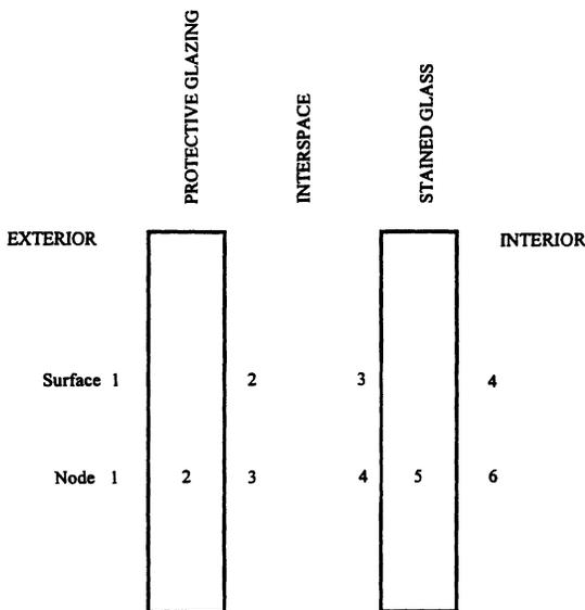
Figure 1 Numbering system for the surfaces and nodes of the glazing system.
