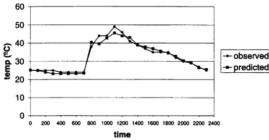
Figure 5 Observed versus predicted temperatures for unvented protective glazing.
