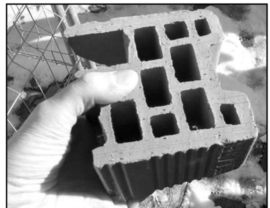
Locally produced building blocks from Marzabotto are energy saving, cheap and require minimum transport
