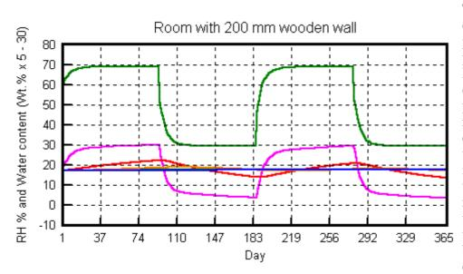
The first graph confirms the prediction in the previous section. Massive wood simply doesn't have the porosity to absorb or release water fast enough to ameliorate the climate. Note that in this graph the upper line is the relative humidity of the room air, while the bunch of lines below is the water content at various
