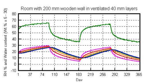
Now there is a good balance between water capacity and the rate of release of water through the surface. The wall has a very marked stabilising effect, giving the interior climate a half time to equilibrium of about two weeks.
