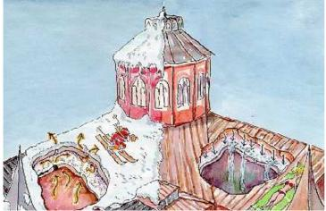
On a warm spring day (the right half of the picture) bright sunlight warmed the dark lead roof to over 80C. Water evaporated from the saturated upper plywood. The vapour diffused through the insulation and condensed on the vapour barrier. The hydrophobic vapour barrier collected the water in drops on its gently sloping surface. At a critical moment two drops coalesced, collected a third and started a little stream down the surface of the polyester. The stream
