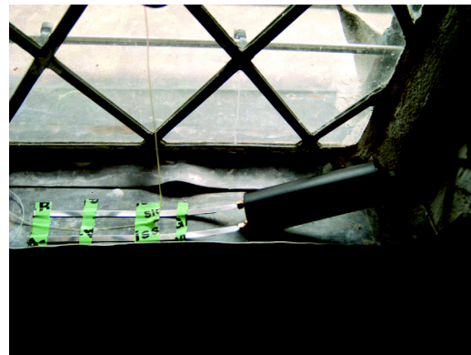
Figure 5 Sensor for humidity on the lead tray.
