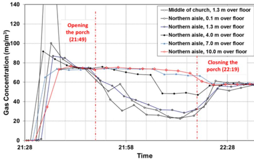
**Figure 3** Tracer gas measurement in the main hall of Hamrånge church.
