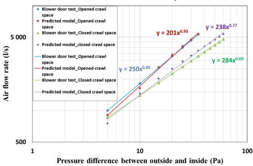
Figure 2 Blower door results for two cases: the apertures of the crawlspace are opened or closed. Power law relationship between pressure difference (x) and airflow rate (y) are presented for each case.
