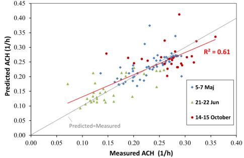
Figure 3 Predicted (simulated) and measured infiltration rates during 5-7 May, 21-22 June and 14-15 October.
