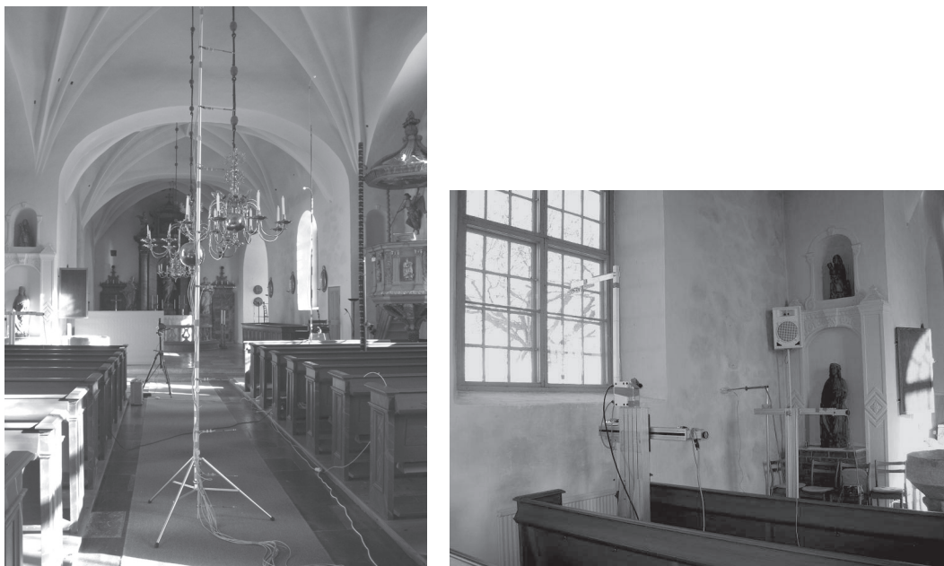
Fig. 4. Anemometer set-up: Hot-sphere (left) and Sonic (right).
